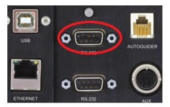
Upgrades FROM P01-13 and earlier cannot be done through the USB or the lower serial port. If you are upgrading from P01-13 or earlier, a dialog box will ask you to confirm that you are using the upper RS-232 (COM) port.
